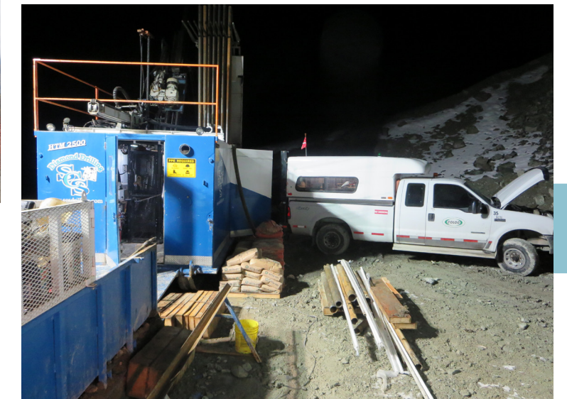
24 hr Geotechnical Well monitoring install and Piezometer
